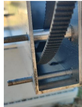
Image showing example of a belt passing ABOVE the lowest bolt.
